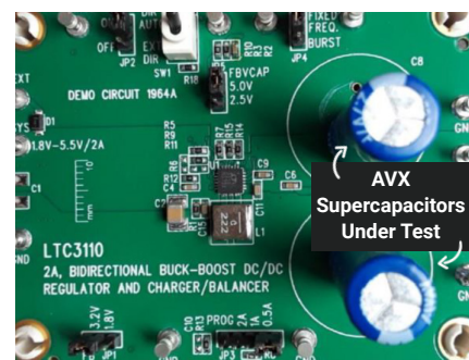
Figure 4: DC1964A Demo Board Based Upon LTC3110 2A, Bidirectional Buck-Boost DC/DC Regulator and Charge/Balancer
