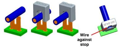
The wire is placed over the slot and the cap loaded onto the contact. On wire stop style caps check that the wire is against the internal stop face.
