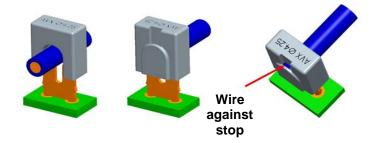
2. The wire is pushed through the gap between the cap and contact. On wire stop style connectors check that the wire is against the internal stop face.
