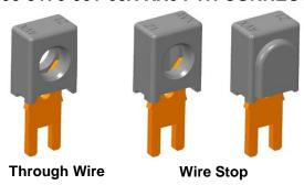
Connector available as a single part in 4 sizes for 18AWG, 20AWG, 22AWG and 24AWG wires. Through wire allows complete flexibility to position the connector anywhere on a wire. Wire stop caps form a stop face for the wire end and protect the wire end after assembly.
