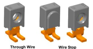
Connector available as a single part in 4 sizes for 18AWG, 20AWG, 22AWG and 24AWG wires. Through wire allows complete flexibility to position the connector anywhere on a wire. Wire stop caps form a stop face for the wire end and protect the wire end after assembly.
