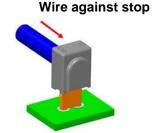
2. The wire is pushed through the gap between the cap and contact. On wire stop style connectors check that the wire is against the internal stop face.
