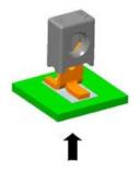
1. It is important to support the underside of the PCB during the assembly procedure.
