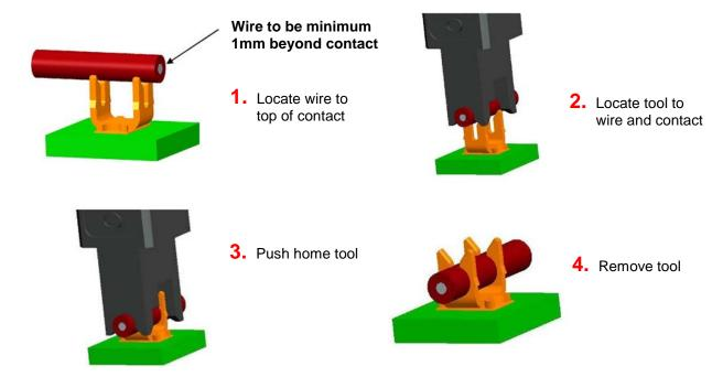
Typical insertion force is approximately 175N per wire for -400 series and 225N per wire for -500 series. This is dependent on the wire gauge, conductor strands and insulation material.
