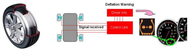
Figure 1: Tyre pressure monitoring system block diagram
