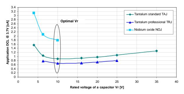
Voltage derating effect on application DCL (C = 47 uF)
