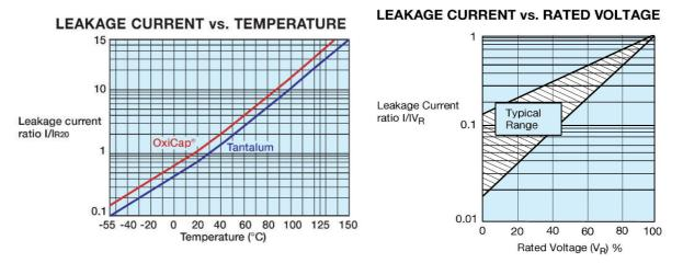
Figure 3: Temperature dependence of DCL
