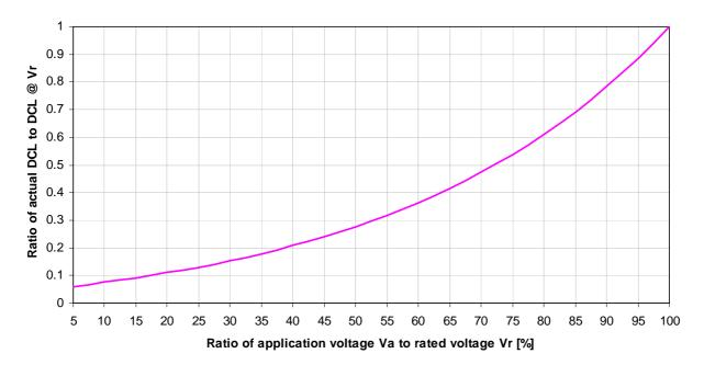
Median DCL ratio vs. Voltage derating
