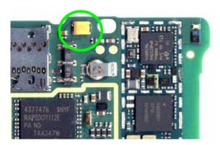
Figure 1: Battery circuit tantalum capacitor in handheld device
