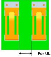
UL approval based on 3.2mm gap between pads, contact centre spacing 5.9mm.
