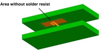
A single pad plated with gold over a nickel under-plate is recommended for good contact under all conditions. Dimensions of pad refer to sales drawing. An area around the mating pad approximately 0.5mm wide should be free of solder resist. This prevents the contact nose riding up on the resist and loosing contact with the pad, see also section 4.2 on misalignment above.
