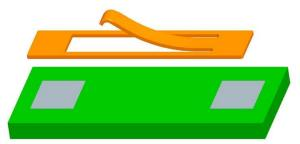
2 solder pads, refer to sales drawing for dimensions. Placing a pad between these is not recommended as it may affect contact performance.
